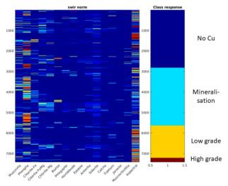
CoreSmart provides deep learning based tools for the information enrichments and management of existing drillhole data. The system is using hyperspectral drillcore scans and an existing database for different mineralization to predict key geochemical properties for the whole core. In detail the system provides:
